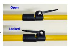
2. Extend the top section of the pole by about 60cm and slide on the yellow clamping float (this is not usually required for the 5m pole). Slide the float down the pole, blue end first with the locking collar towards to the top of the pole. Tighten the collar until the float remains firmly in place
